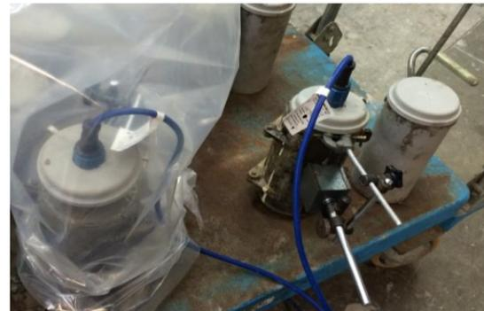
Figure 1: pH sensors embedded in GPC cylinders
