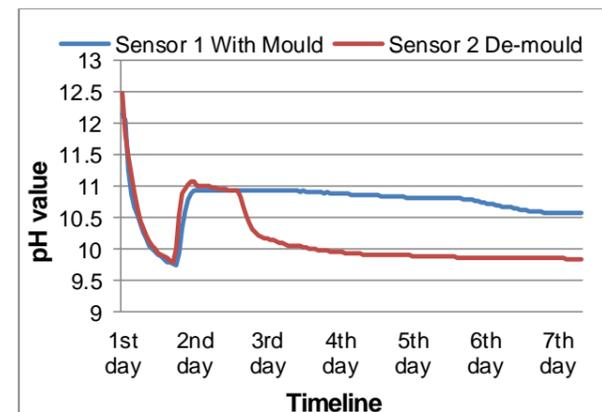
Figure 2: pH value during curing process
