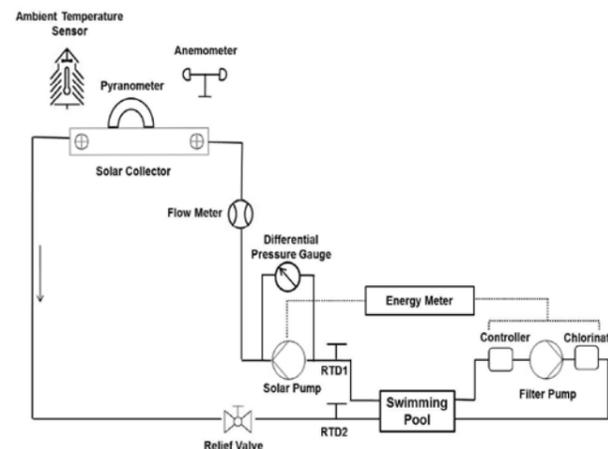
Figure 3: New Pipe Work and Data Logging System
