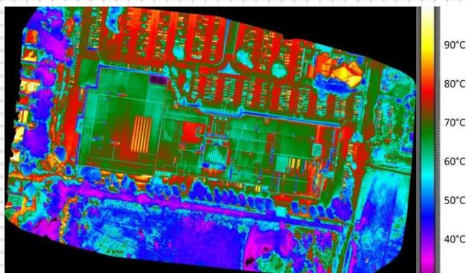
Figure 3: Thermal image looking down at one of the case study buildings, with a metallic coated steel roof.
