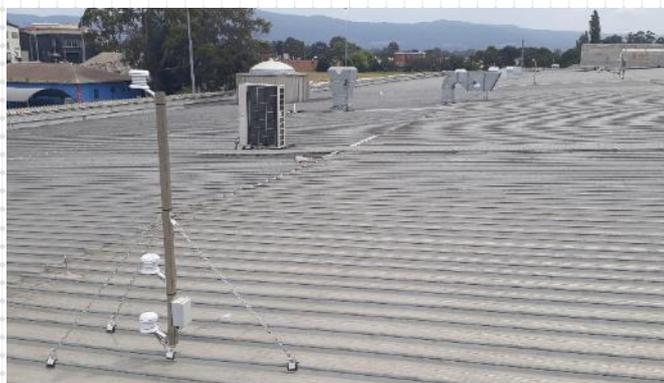
Figure 2: Detailed mapping of air and surface temperatures above the case study buildings using 15 environmental sensors.
