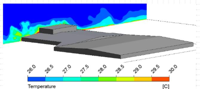
Figure 1: Simulated temperature field above a shopping centre roof.
