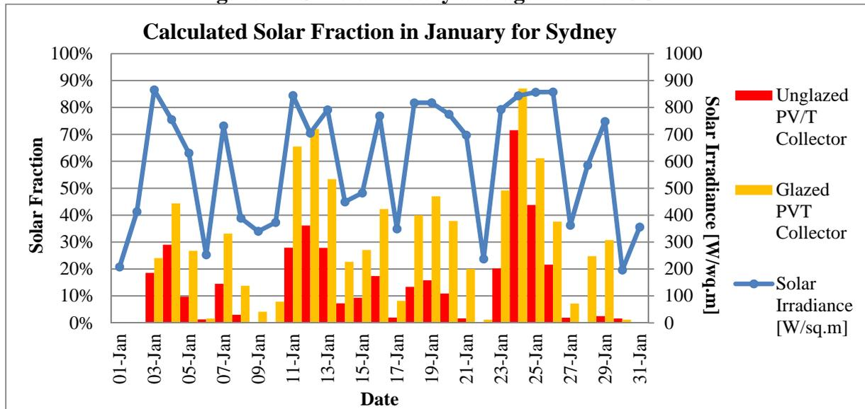
Figure 8 – Simulated daily average solar fraction
