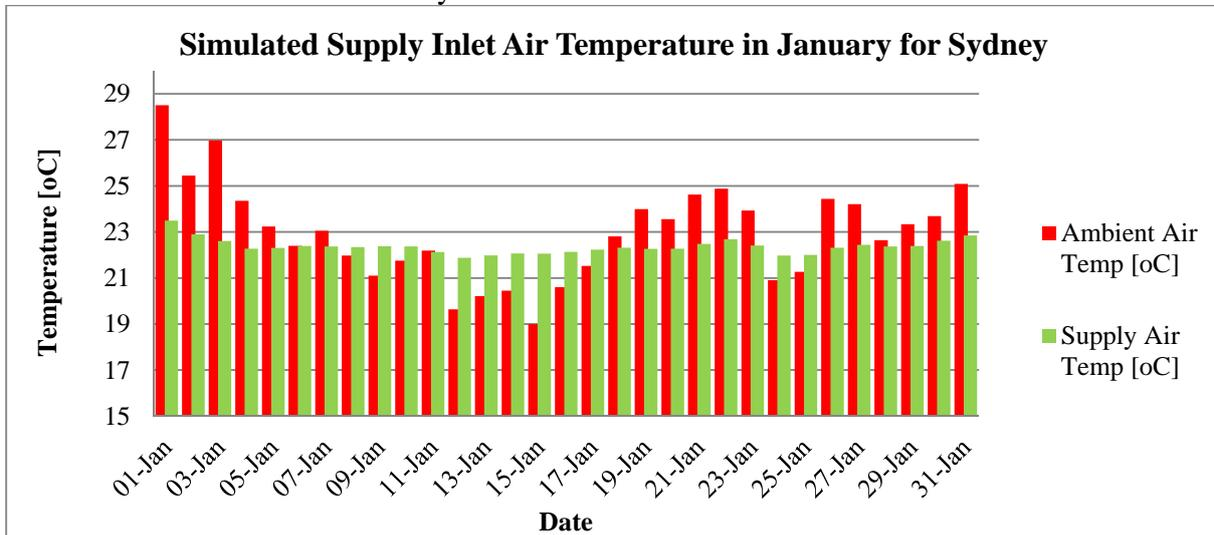
Figure 6 – Simulated daily average supply air temperature outlet
