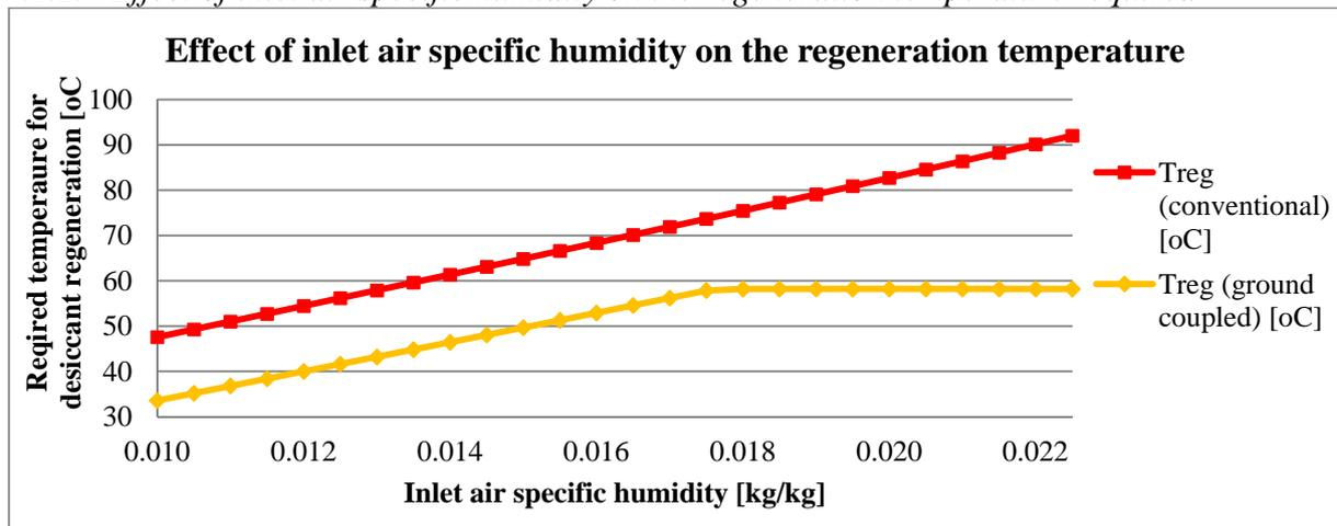
**Figure 4 – Effect of inlet air specific humidity on the regeneration temperature (ground coupled vs. conventional)**
