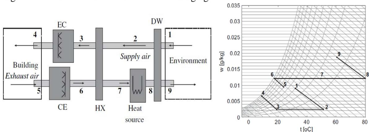
**Figure 1 – A conventional desiccant air cooling cycle schematic (left) and psychrometric process (right) (Panaras et al., 2010)**
