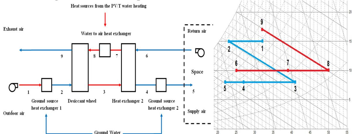
**Figure 2 – Ground coupled PV/T desiccant air cooling cycle schematic (left) and psychrometric process (right)**
