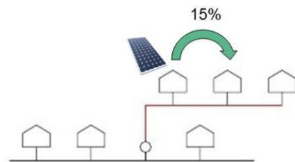
Figure 2. Schematic diagram of an embedded network. The top three houses are on an embedded network. The circle represents the common connection point to the public distribution network.
