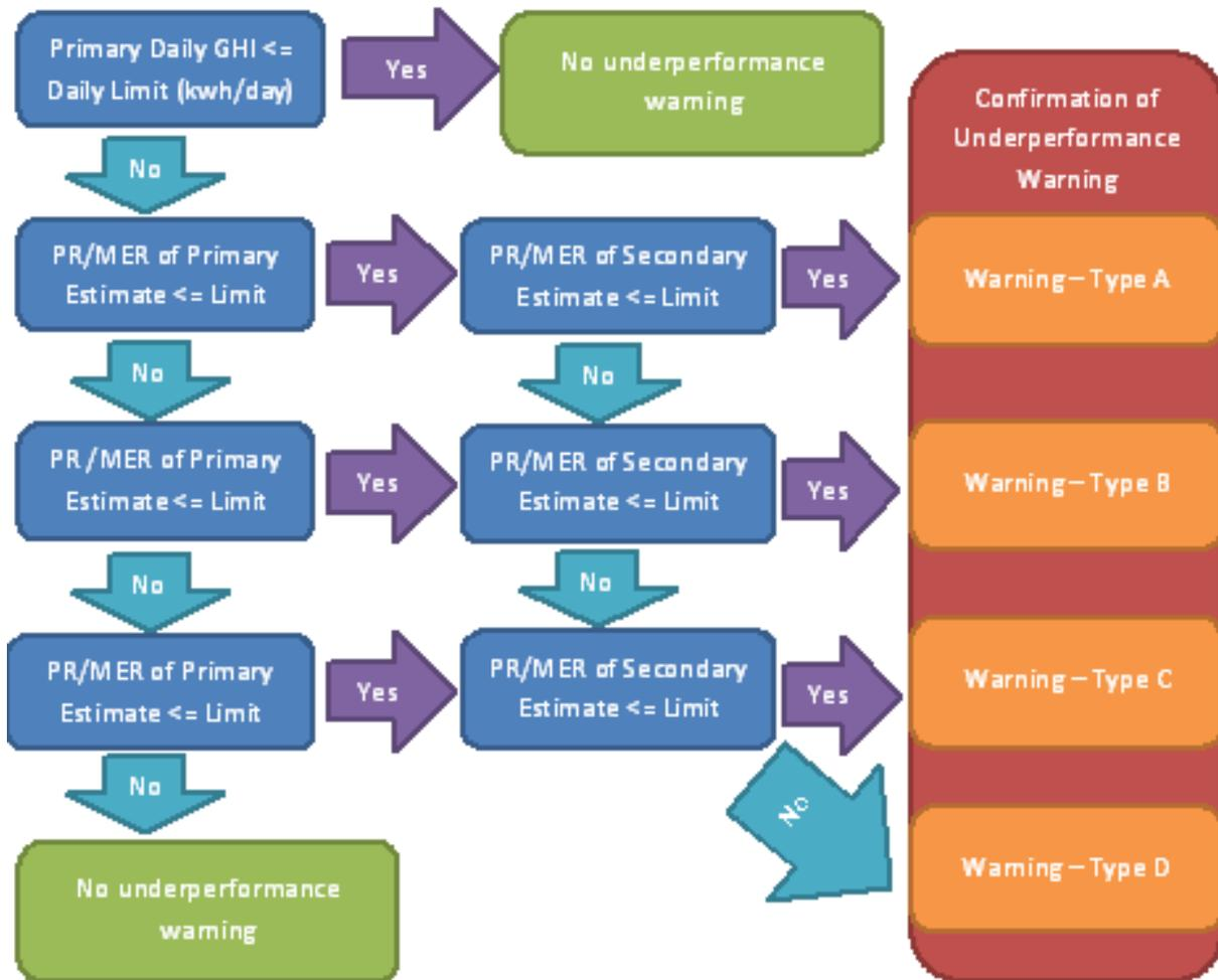
Figure 8 Process flow for diagnosis of underperformance based on the daily level
