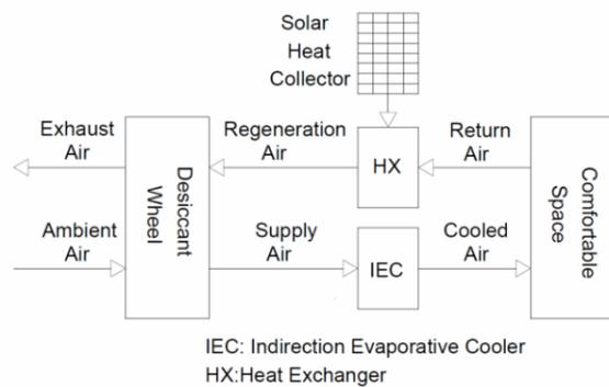
Figure 1: Schematic diagram of a desiccant-IEC air conditioning system
