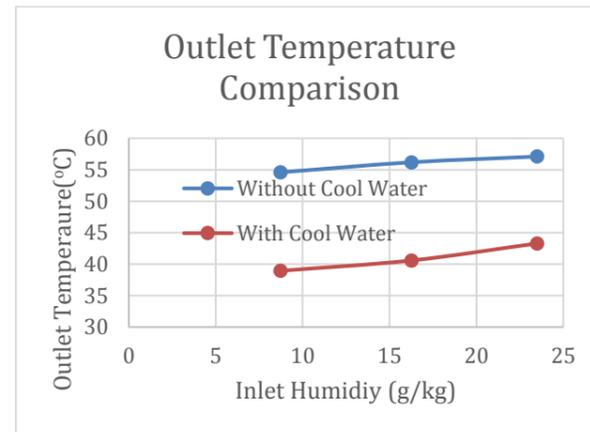
Figure 3: Outlet temperature comparison between conventional wheel and internal cool wheel
