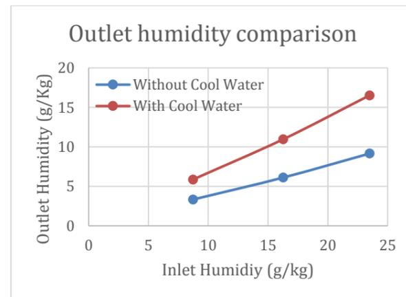
Figure 2: Outlet humidity comparison between a conventional wheel and internally cooled wheel
