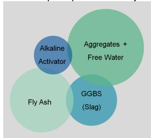
Figure 1: Geopolymer concrete constituents
