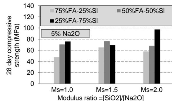
Figure 2: 28<sup>th</sup> day compressive strength of geopolymer mortar samples
