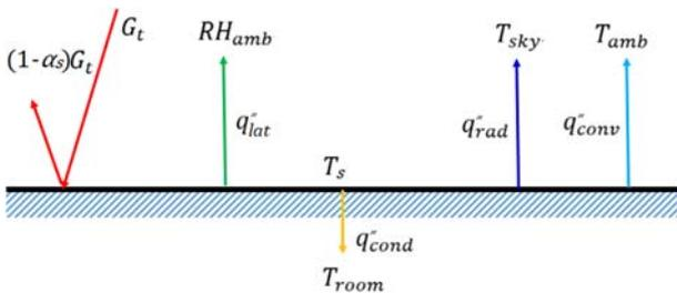
Figure 3: Energy balance of a flat roof.
