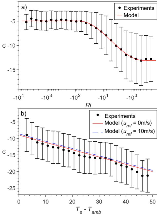
Figure 12: Comparison of the thermal boundary layer shape parameter,  $\alpha$ , obtained from experimental data with those predicted by the above-roof temperature model, in a) stable and b) unstable conditions. Experimental data has been represented by the mean (dot) and standard deviation (whiskers) of  $\alpha$  within discrete bins.
