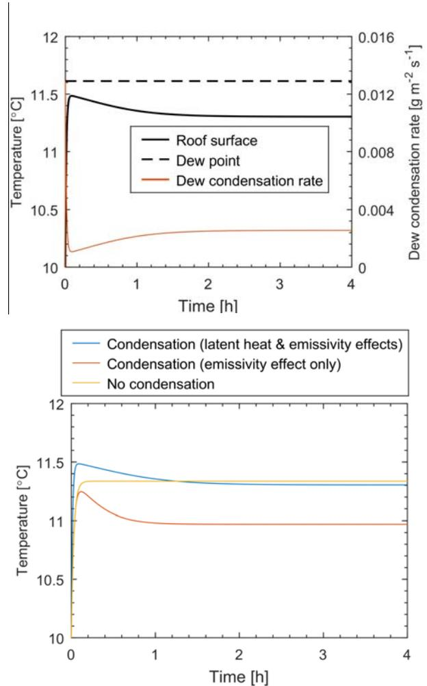
Figure 7: Modelling results for Baseline case: a) for roof surface temperature, and b) for comparison of the roof surface temperatures considering different effects.
