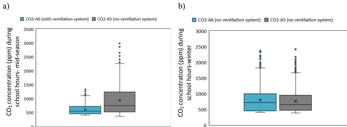
Figure 5: Box plot of CO<sub>2</sub> after (a) and before (b) installation of the ventilation system
