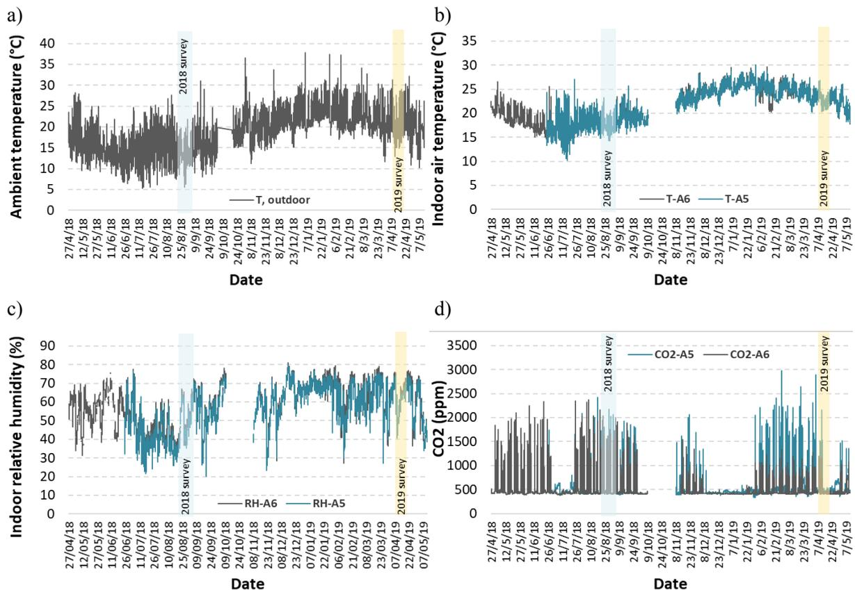
Figure 4: Results of monitoring during cold and mid-season: outdoor temperature (a), indoor air temperature (b), indoor relative humidity (c), CO<sub>2</sub> (d) in A6 (classroom with ventilation system) and A5 (classroom without ventilation system)
