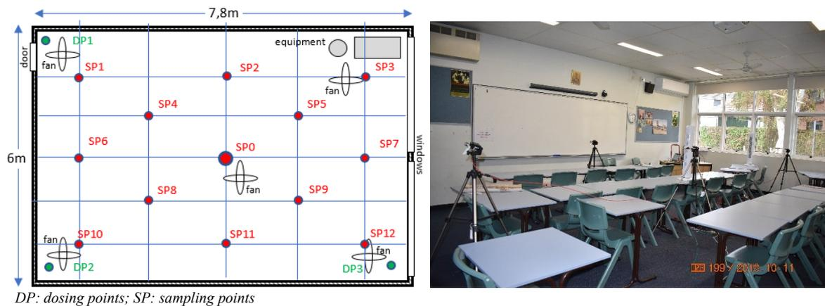
Figure 3: Tracer gas measurement
