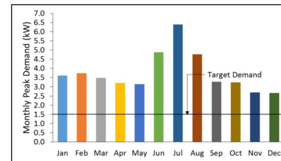
Figure 2: Monthly Peak Demands with 2.5 kW<sub>p</sub> PV and without Battery.
