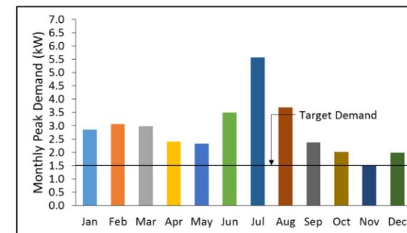
Figure 4: Monthly Peak Demands Using CS4 with 2.5 kW<sub>p</sub> PV and 1 kWh Battery.
