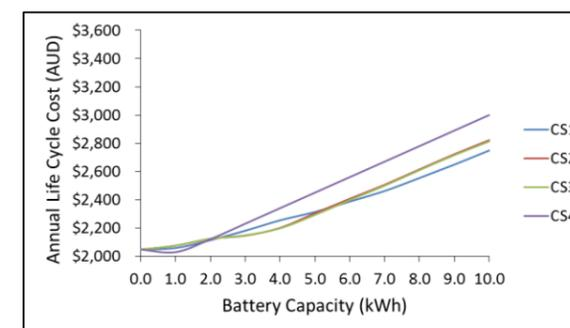
Figure 6: Life Cycle Cost of Electricity with 2.5 kW<sub>p</sub> PV.
