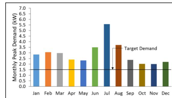
Figure 3: Monthly Peak Demand Using CS4 without PV and with 1 kWh battery.
