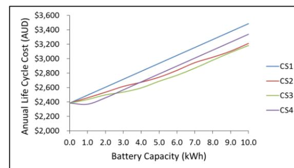
Figure 5: Life Cycle Cost of Electricity without PV.
