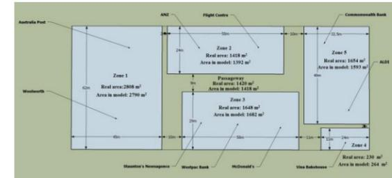
Figure 4: Dimensions of the shopping centre model established.
