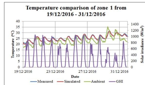
Figure 3: Measured and simulated temperature comparison.
