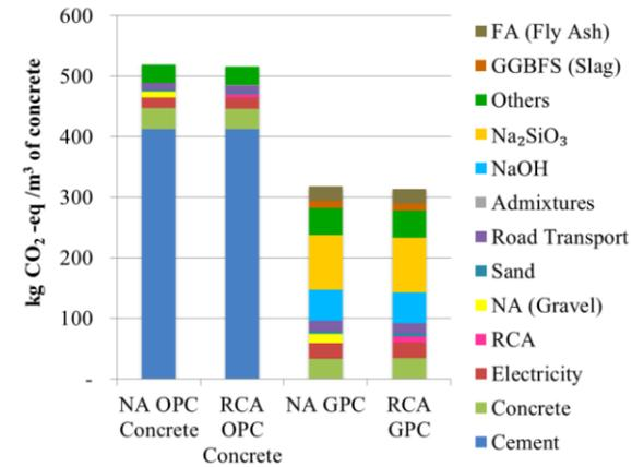
Figure 3: CFI of two types of concrete investigated with either NA or a 100% replacement with RCA
