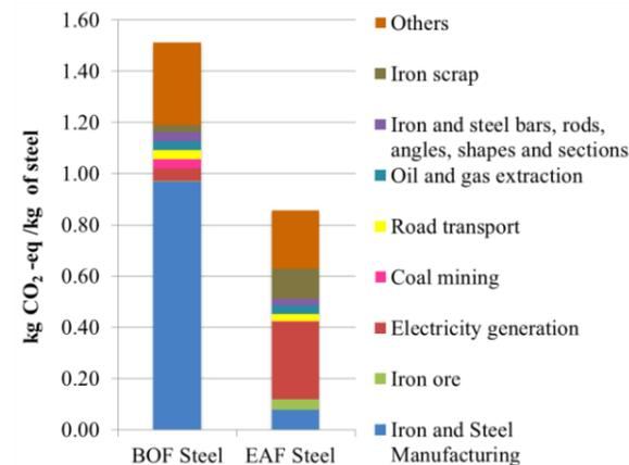
Figure 4: CFI of two types of BOF and EAF steel with the use of iron and steel scrap investigated
